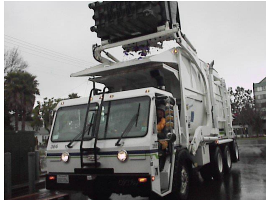
A City of Berkeley front-end loader truck emptying a customer's food scraps.
